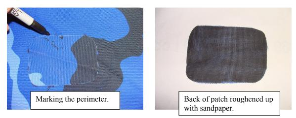
3. Spread a thin layer of adhesive around the hole to be patched. Lay patch over the adhesive and press firmly together. The adhesive is very runny so use it carefully. Adhesive dries in about 3 minutes and is fully cured in about 15 minutes.
